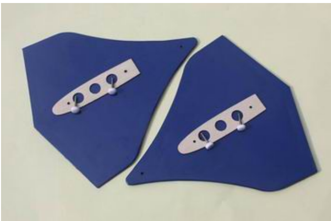
Side force generators (mounted with four M3X18 hand bolts and 2 balsa sheets)
